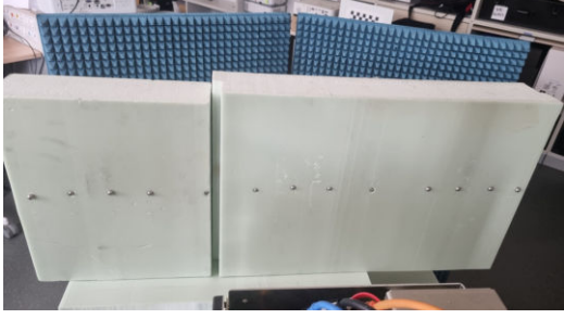
Fig. 9. Styrofoam board with mounted metal spheres of \varnothing 1 cm.
